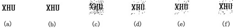
Fig. 4. Experiment results for resist attacking. (a) Echo; (b) Blow-up/Reduce; (c) Resampling; (d) MP3 compress; (e) Lowpass; (f) Gaussian white noise.
